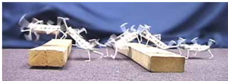
Figure 4.6 – Composite of video frames showing Mini-Whegs 5 traversing two 3.8cm by 8.9cm obstacles while running at three body lengths per second.
