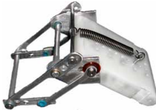
Figure 2.14 – The Four-bar jumping mechanism is powered by a linear extension spring on top of the robot.
