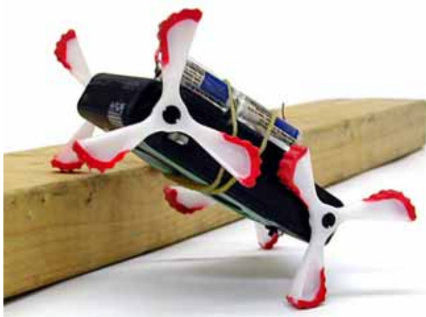
Figure 6.6 – The robot is able to surmount the 3.8 cm obstacle.
