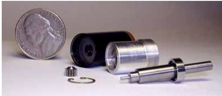
Figure 3.4 – Custom components for the jumping transmission in Mini-Whegs 4J: (clockwise from nickel shown for scale) Maxon 275:1 planetary transmission, custom shaft housing, custom input shaft, clip to hold shaft in place, input gear for transmission.
