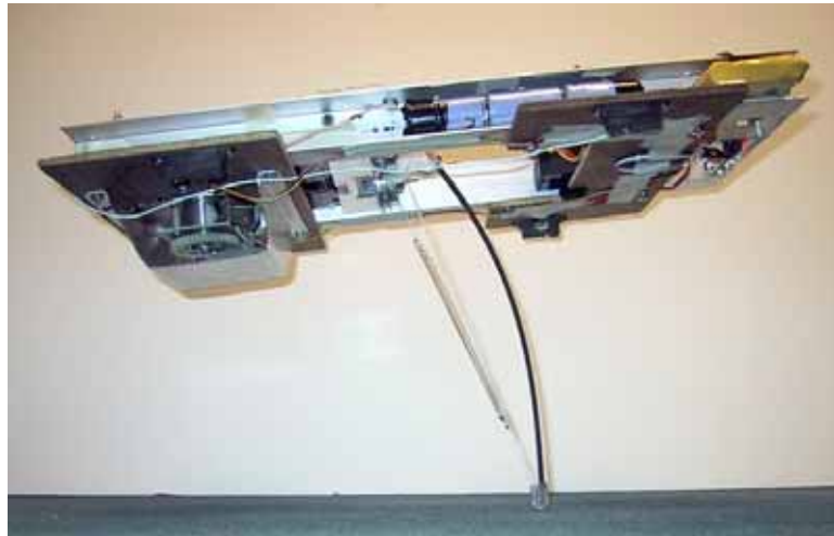
Figure 2.10 – A single flexible fiberglass leg adjusted by control strings forms the propulsion method for the 3D Bow Leg Hopper.
