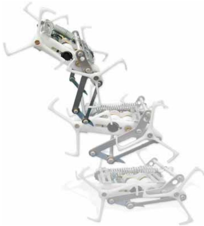
Figure 3.5 – Photographs illustrating the motion of the four-bar mechanism during a jump.
