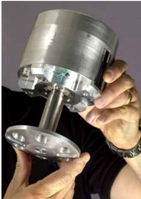
Figure 2.8 – The Hopper can leap up to 6 meters high using a gasoline combustion powered piston.
