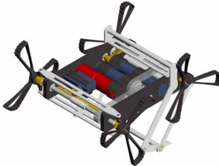
Figure 5.3 – Rendering of the complete Pro/ENGINEER model of Mini-Whegs 6J.
