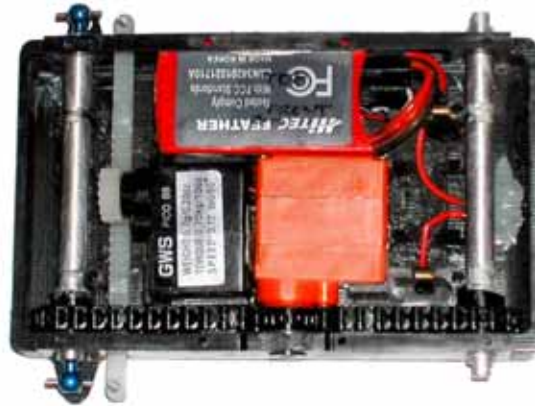
Figure 6.1 – Photo of the interior of Mini-Whegs 7, showing the single drive chain, wheg axles, servos for drive and steering, and radio receiver.
