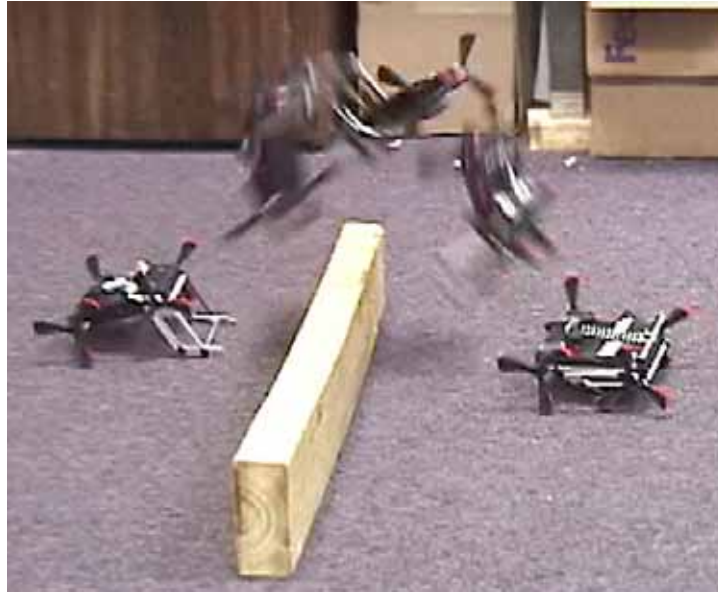
Figure 7.5 – Composite of video frames showing Mini-Whigs 9J easily clearing a 9cm barrier.
