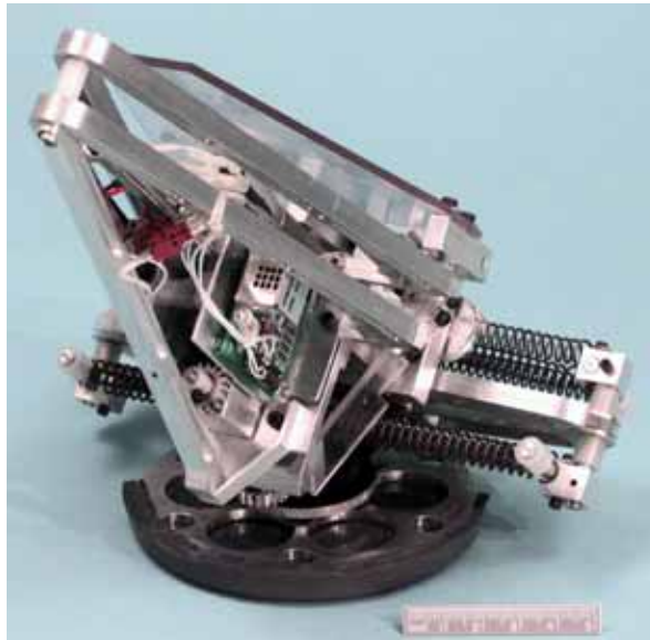
Figure 2.9 – Stiff springs contract quickly to extend the bent leg of Froghopper.
