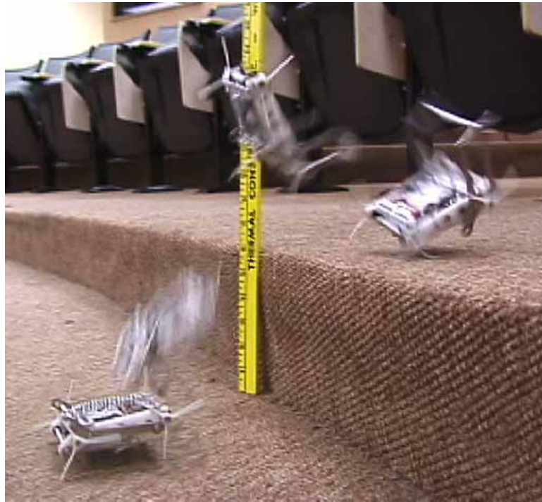
Figure 3.7 – Composite of video frames showing Mini-Whegs 4J jumping up a 15cm stair.
