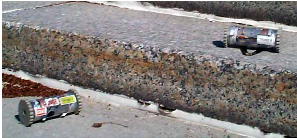
Figure 2.7 – Scout includes a triangular spring steel jumping foot which allows it to jump up stairs.
