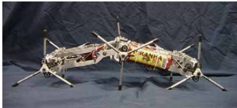
Figure 2.5 – Whogs II incorporates a body joint for increased mobility.
