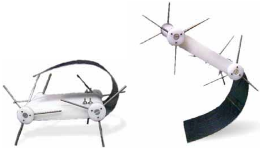
Figure 2.12 – The Scorpion jumping concept retracted on top of the robot before a jump (left), and then released from the bottom of the robot (right).
